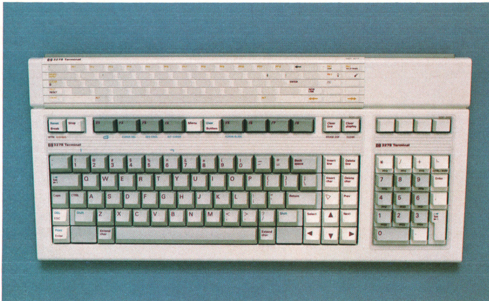
Fig. 3. Overlays for the numeric and function keys and a reference plate for the main array can be used to relabel keys that are redefined by specific applications.
