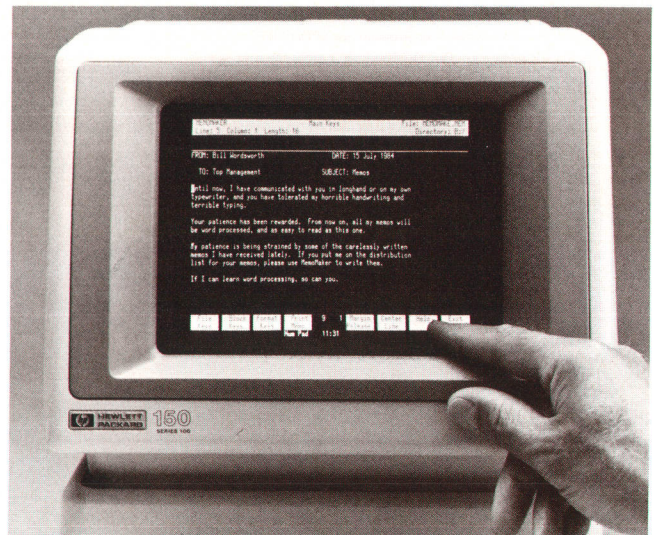
Fig. 3. The green-phosphor CRT displays 24 80-character rows of text, plus three rows of status and softkey information.
