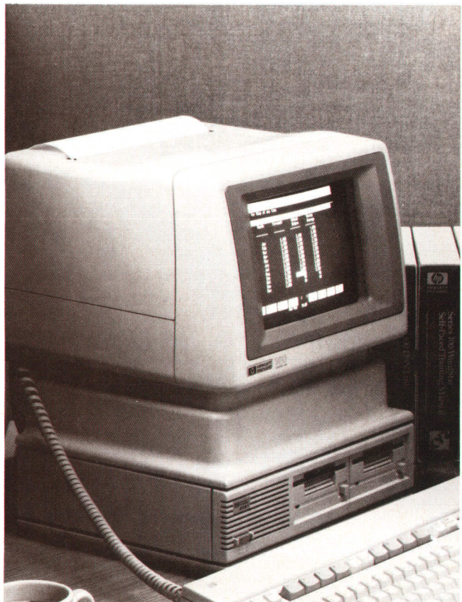
Fig. 1. The 2674A Printer is a thermal printer that fits into the top of the HP 150 Personal Computer cabinet.
